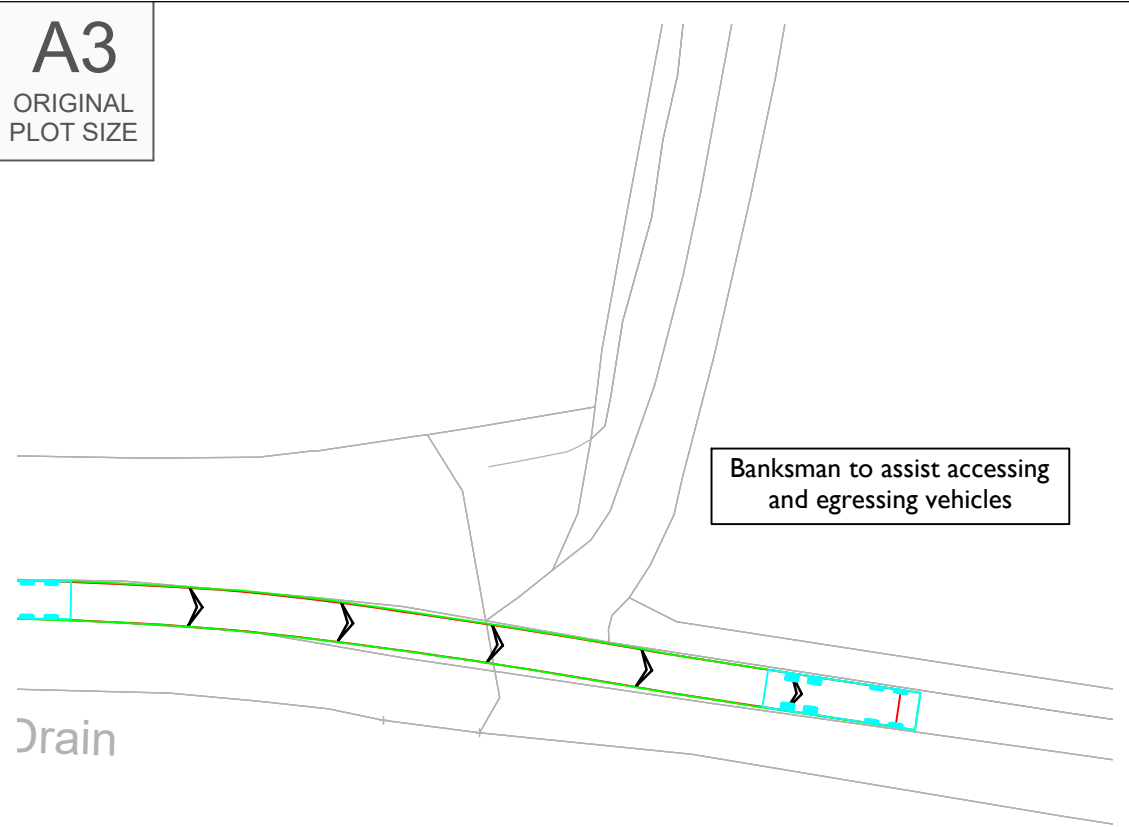
Tipper Vehicle Entering Site
